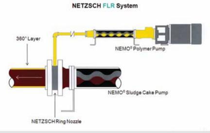
NETZSCH Friction Loss Reduction system
